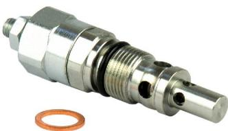
The main relief valve is fitted in a M20x1.5 cavity and is built with a guided poppet to improve pressure setting stability and avoid the typical noise of lower cost alternative valves
