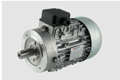
**B14 motors:** for market compatibility, any standard B14 AC motor with frame 71, 80, 90 or 100/112 can be mounted. In this case two-pieces couplings and additional adaptor flanges as per tables U040.40.10, .11, .12 and .13 must be mounted.
