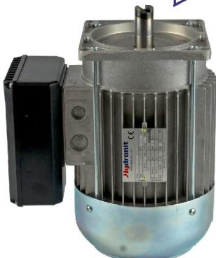
**B14 standard AC motors:** the standard solution easily available on every market from 0,25 to 7,5 kW, single or three phase. These motors are normally procured by the customer itself. Hydronit provides adaptor flanges and double piece coupling for frame size: 71, 80, 90, 100 and 112.
