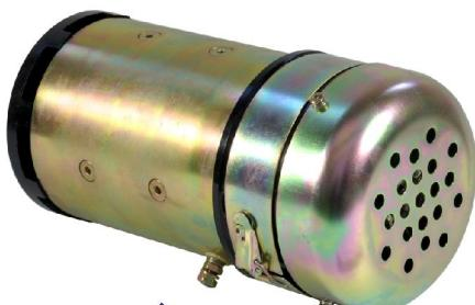
**Frame 151 DC motors:** real heavy duty bulk motors, with fan cooling, thermal protector and running time up to 16 min or over. Power from 2,5kW 12VDC up to 4kW 24VDC.
