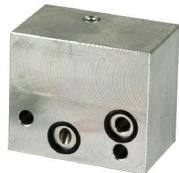
Piloted operated check valves can be integrated within a modular manifold block for Ng6 (cetop3) valves, thus avoiding the extra modular cetop 3 sandwich type valve between the base block and the spool valve.
